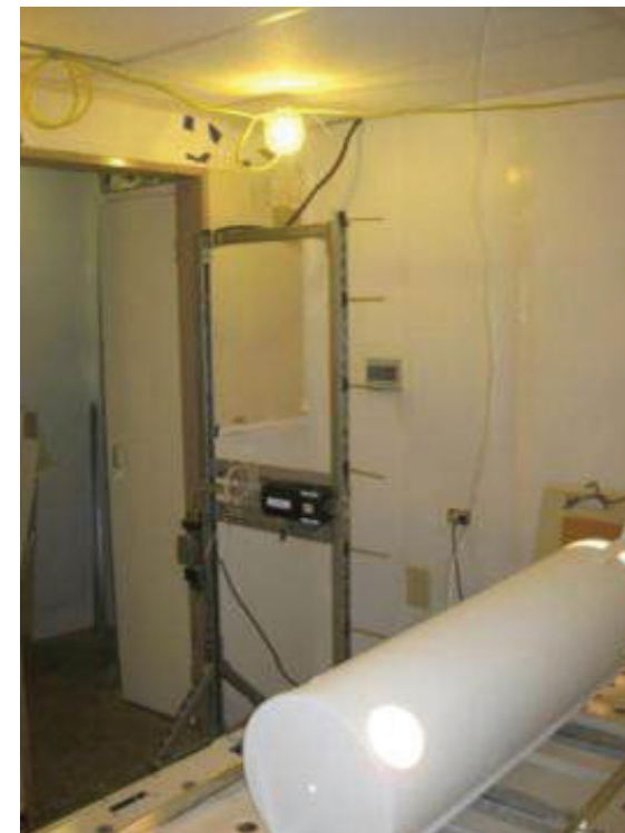
Above and left: the Maricopa Health Clinic uses displacement ventilation. The process of deciding to deploy that system included computer modeling of airflow, as well as real-world mock-ups to test the system in an actual space.
